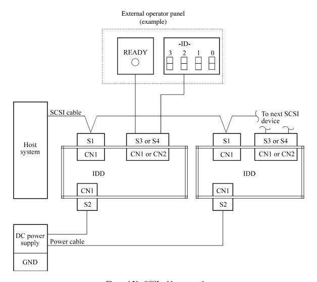
Figure 4.20 SCSI cables connection
